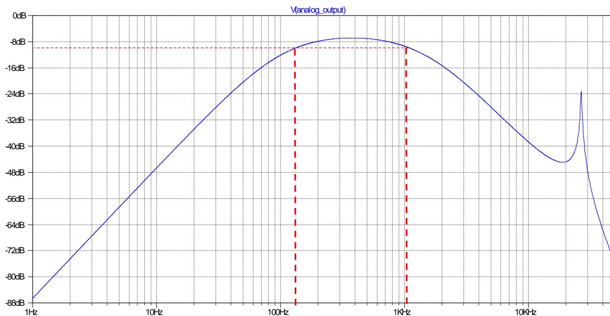
Fig 10. Frequency Response Curve of PKGX-14-4010
