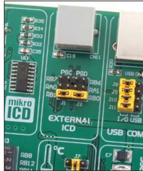
Figure 5-2: Pins RB0 and RB1 are used for programming
