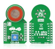
CO click<sup>™</sup> is a simple solution for adding a high-sensitivity Carbon monoxide sensor to your design. The board features an MQ-7 sensor with a SnO2 gas sensing layer, a calibration potentiometer, a **mikroBUS**<sup>™</sup> host socket, two jumpers and a power indicator LED. CO click<sup>™</sup> communicates with the target board through mikroBUS<sup>™</sup> AN (OUT) line. CO click<sup>™</sup> is designed to use a 5V power supply only.
