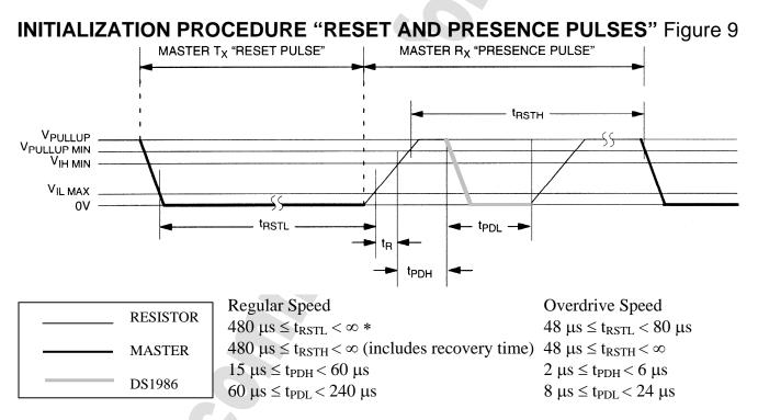
In order not to mask interrupt signaling by other devices on the 1-Wire bus, t<sub>RSTL</sub> + t<sub>R</sub> should always be less than 960 µs.
