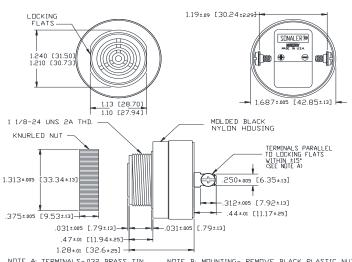
NOTE A: TERMINALS-032 BRASS TIN PLATED, TAPPED FOR #6-32 SCREW, TWD #6-32 NICKEL PLATED BRASS SCREWS INCLUDED, WILL ACCEPT 1/4\* QUICK CONNECT. NOTE B MOUNTING- REMOVE BLACK PLASTIC NUT
