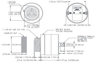
NOTE A: TERMINALS-.032 BRASS TIN PLATED, TAPPED FOR #6-32 SCREW. TWO #6-32 NICKEL PLATED BRASS SCREWS INCLUBED. WILL ACCEPT 1/4\* QUICK CONNECT. NOTE B: MOUNTING- REMOVE BLACK PLASTIC NUT AND INSERT THREADED FRONT THROUGH 1.25' HOLE PUNCHED IN PANEL, IF DRIENTATION IS NEEDED, NOTE LOCKING FLATS ON DRAWING. SCREW NUT BACK ON. DO NOT DVERTIGHTEN.
