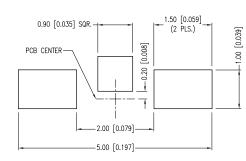
\*UNLESS OTHERWISE SPECIFIED TOLERANCES PER DECIMAL PRECISION ARE: X=±1 (±0.039), X.X=±0.5 (±0.020), X.XX=±0.25 (±0.010), X.XXX=±0.127 (±0.005). LEAD SIZE=±0.05 (±0.002), LEAD LENGTH=±0.75 (±0.030). MIN=  $^{+0.00}_{-0.00}$  MAX.=  $^{+0.00}_{-0.00}$ UNCONTROLLED DOCUMENT
