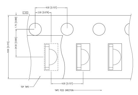
\*UNLESS OTHERWISE SPECIFIED TOLERANCES PER DECIMAL PRECISION ARE: X=±1 (±0.039), X.X=±0.5 (±0.020), X.XX=±0.25 (±0.010), X.XXX=±0.127 (±0.005). LEAD SIZE=±0.05 (±0.002), LEAD LENGTH=±0.75 (±0.030). MIN= +DECIMAL PRECISION MAX.= +0.00 (±0.000), X.XX=±0.127 (±0.000). UNCONTROLLED DOCUMENT
