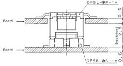
Note: The 2.9mm board to board size does not include the soldering paste thickness.
