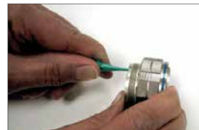
Plastic tool with contact in proper position.
