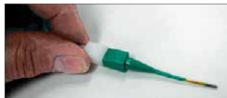
Plastic tool with contact in proper position.
