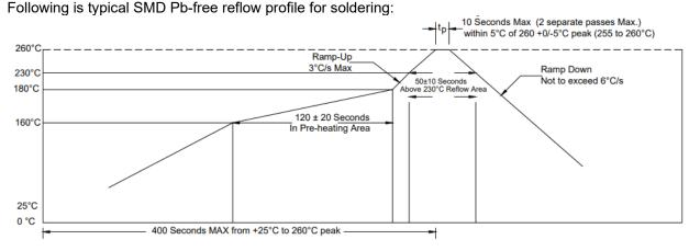
Excessive heating time at high temperature may result in deterioration of the characteristics and may break the crystal unit. For manual rework, heat the lead part at 300°C or lower for 5 seconds or less.
