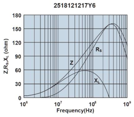
Impedance, reactance, and resistance vs. frequency.
