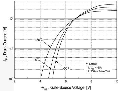
Figure 2. Transfer Characteristics
