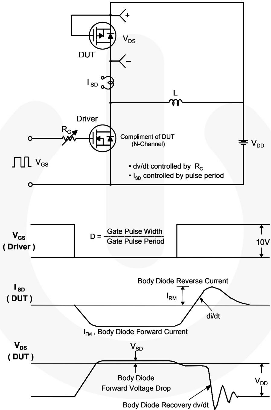
Figure 15. Peak Diode Recovery  $dv/dt$  Test Circuit & Waveforms
