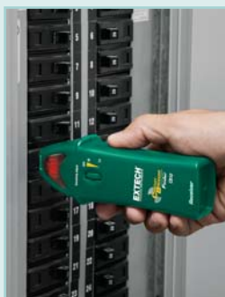
Adjustable sensitivity for pinpointing the correct breaker
