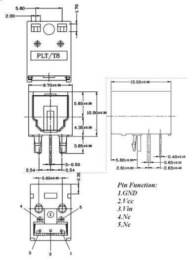
Note: 1.All dimensions are in millimeters. 2.General Tolerance :±0.3mm
