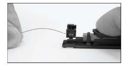
Release the bow in the fiber and fully close the left buffer clamp. Again, you will hear an audible snap.
