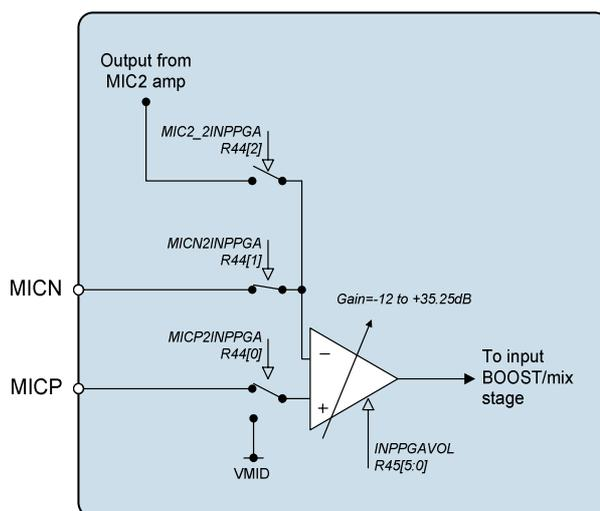
**Figure 6 Microphone Input PGA Circuit**
