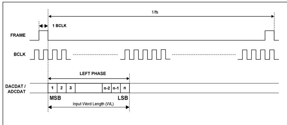
Figure 28 DSP/PCM Mode Audio Interface (mode A)
