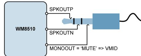
Figure 23 Recommended Headphone Output Configurations
