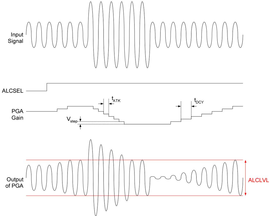
**Figure 11 ALC Normal Mode Operation**
