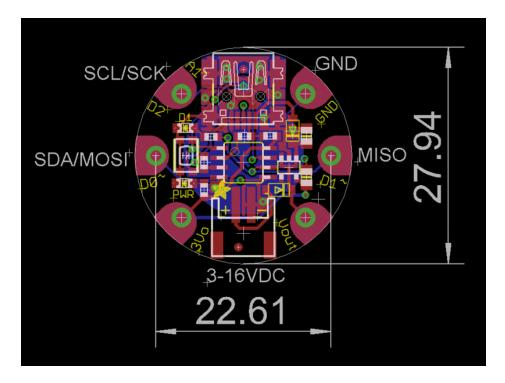
This diagram shows the physical size of the Gemma (diameter in mm) and the distance from pad to pad. The pads are at exact 90 & 45 degree angles except for 0 and 180 which is where the USB/JST connectors go
