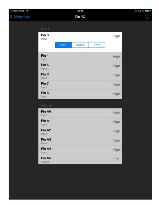
Some of the various options can be seen below, such as the ability to change the PWM rate when you select PWM mode, or whether to set output pins high or low, etc.:
