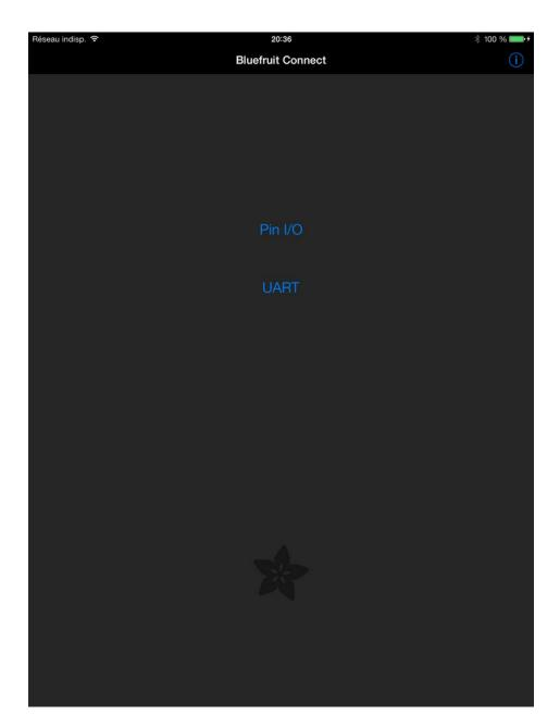
This will establish a connection between the nRF8001 and your iOS device, and you should see an I/O screen that allows you to select any available pin.
