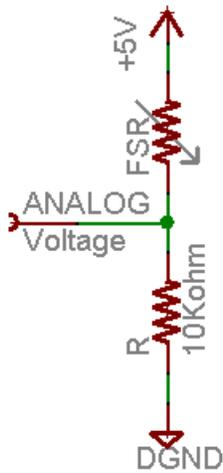
For this example I'm showing it with a 5V supply but note that you can use this with a 3.3v supply just as easily. In this configuration the analog voltage reading ranges from 0V (ground) to about 5V (or about the same as the power supply voltage).
