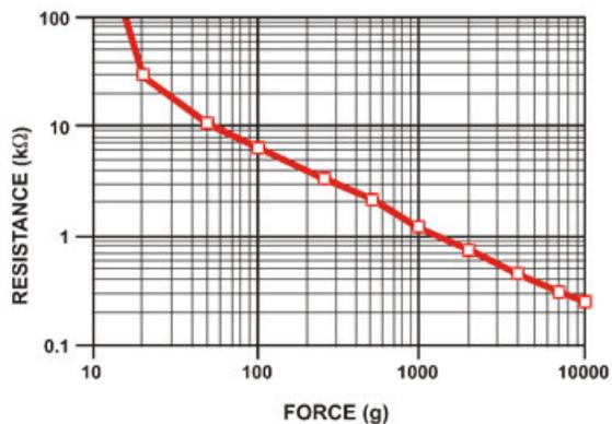
It is important to notice that the graph isn't really *linear* (its a log/log graph) and that at especially low force measurements it quickly goes from infinite to 100K $\Omega$ .
