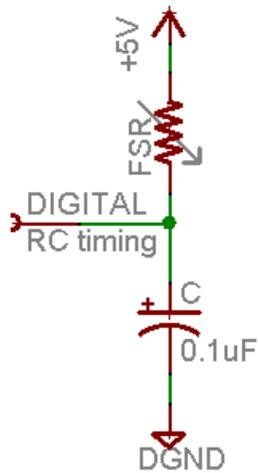
In this case, our 'bucket' is a 0.1uF ceramic capacitor. You can change the capacitor nearly any way you want but the timing values will also change. 0.1uF seems to be an OK place to start for these FSRs.
