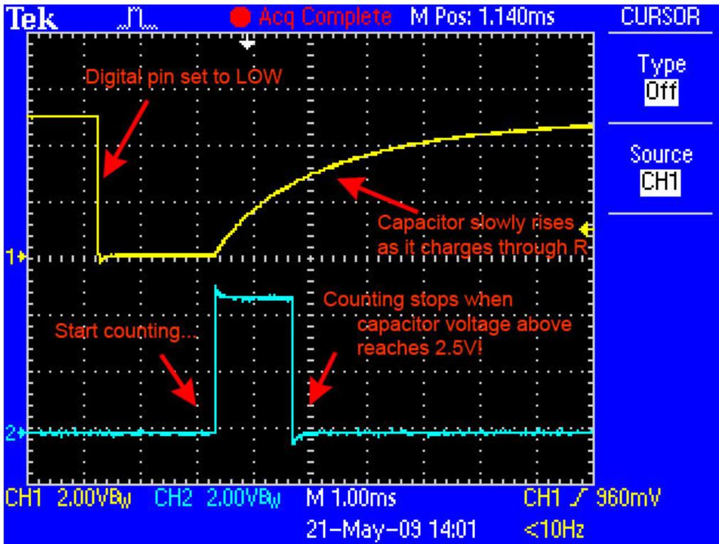
This capture from an oscilloscope shows what's happening on the digital pin (yellow). The blue line indicates when the sketch starts counting and when the counting is complete, about 1.2ms later.
