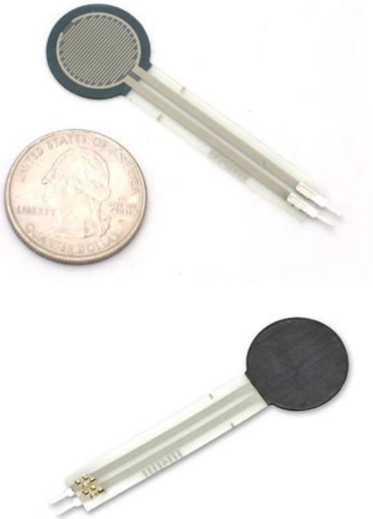
The FSR is made of 2 layers separated by a spacer. The more one presses, the more of those Active Element dots touch the semiconductor and that makes the resistance go down.
