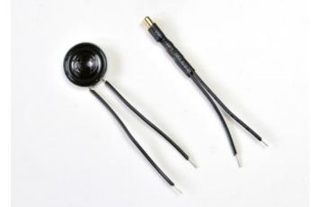
Your speaker and tilt ball switch are now ready for attaching to the rest of your circuit!
