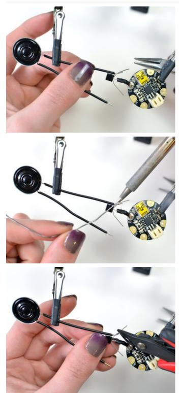
Set up the speaker in your helping hand tool and position one of its wire leads next to the transistor lead on the right.
