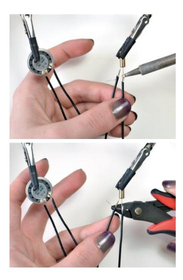
Slide a piece of the smallest diameter heat shrink tubing over each leg of the tilt ball switch to insulate the wires and solder connections.
