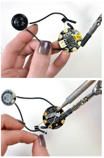
Bend the speaker's other wire to the Vout pin on GEMMA and solder in place.
