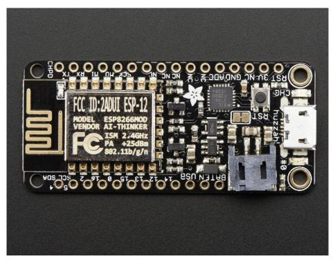
While the Feather HUZZAH ESP8266 comes pre-programmed with NodeMCU's Lua interpretter, you don't have to use it! Instead, you can use the Arduino IDE which may be more familar. This will write directly to the firmware, erasing the NodeMCU firmware, so if you want to go back to Lua, use the flasher to re-install it (https://adafru.it/f1O)
