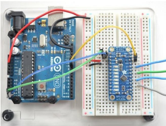
The reset pin is not required for use, but if you can spare a pin, it will make the system a little more rugged - the Arduino will do a hard reset of the CAP1188 on startup, connect **RST** to any digital I/O pin. In the library example code you can set up that pin in the CAP1188 object creation.
