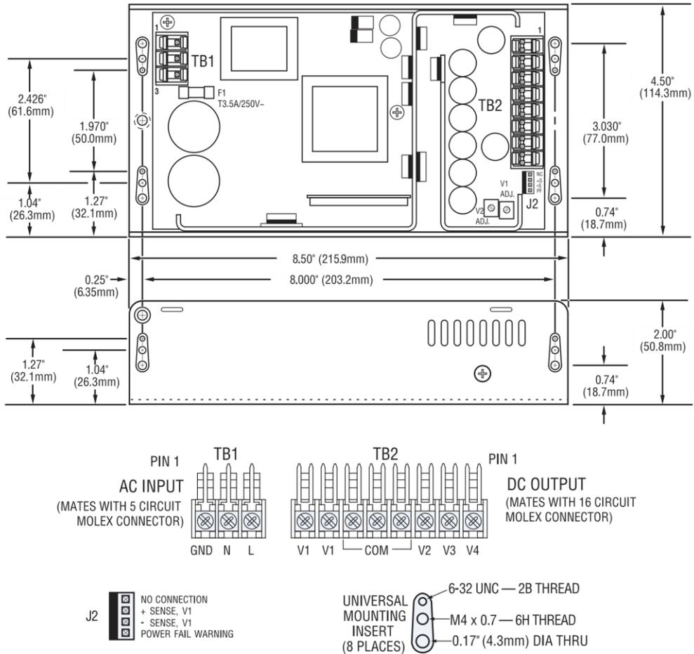
Figure 1. Mechanical Drawing
