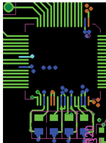
Figure 62. Top Layer Decoupling REFIN/REFOUT, REFCAPA, REFCAPB, and REGCAP Pins
