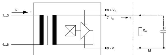
**Possibilities of wiring for V<sub>C</sub> = ±15V** (@ θ<sub>A</sub> = 85°C, R<sub>M</sub> = 22 Ω)
