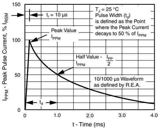
Fig. 3 - Pulse Waveform
