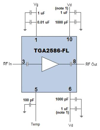
Note 1: These caps can be removed for drain pulsing. Drain volatge must be biased from both sides top and bottom Vd pins-
