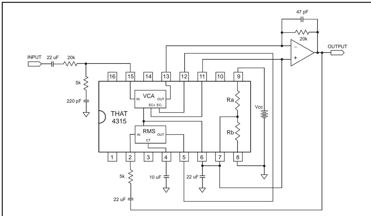
Figure 4. 4315 Typical Application Circuit - 2:1 Compressor
