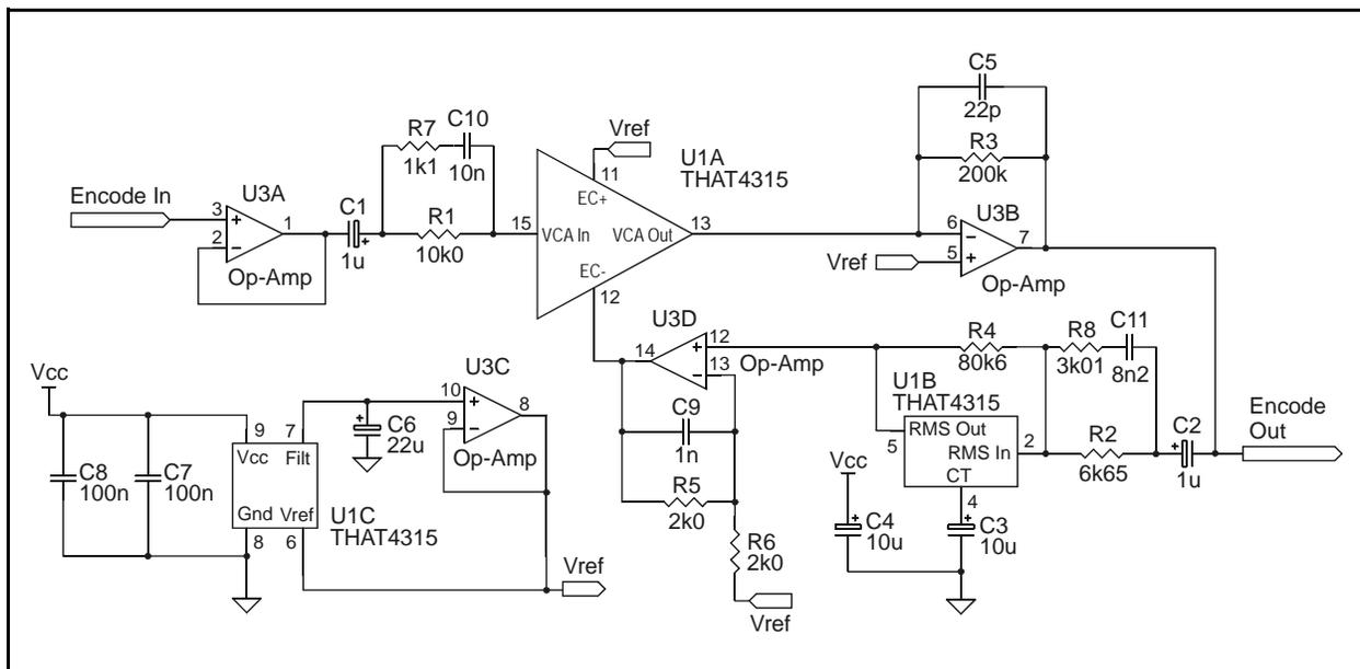
Figure 8. 3:1 Encoder circuit
