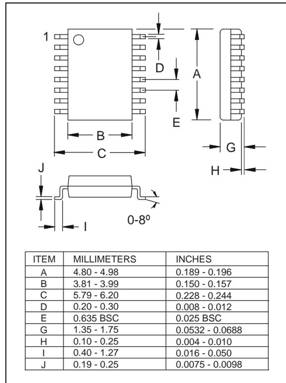
Figure 10. QSOP-16 surface mount package drawing
