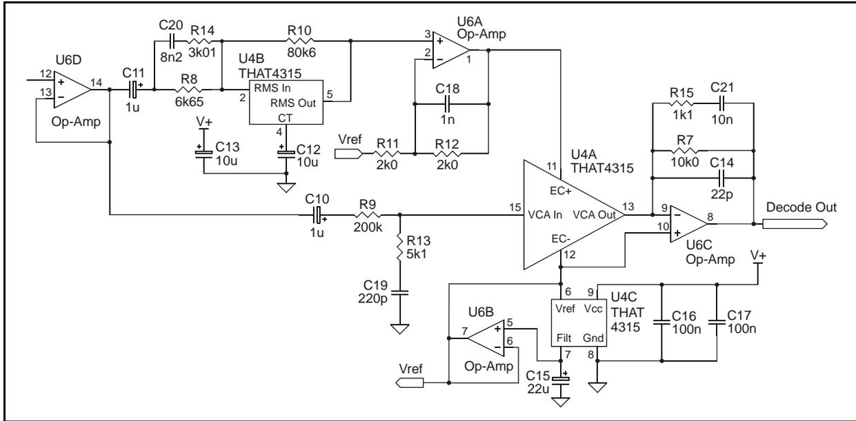
Figure 9. 3:1 Decoder circuit
