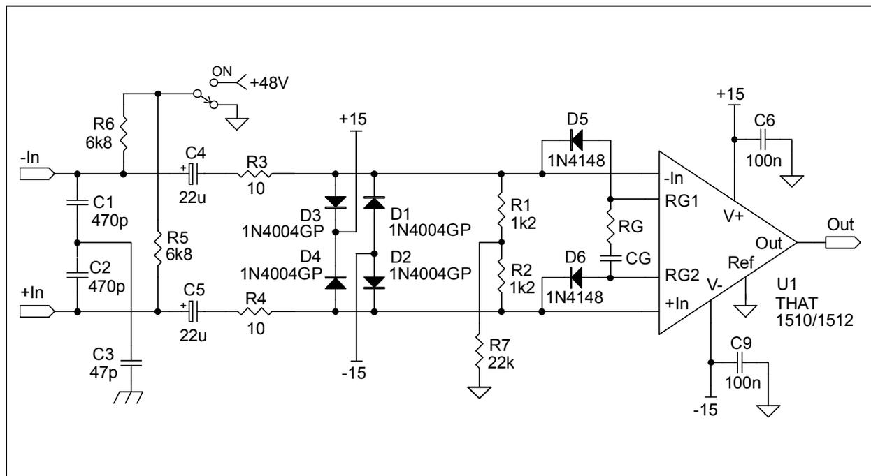
Figure 5. Recommended 1510 / 1512 Circuit with Phantom Power
