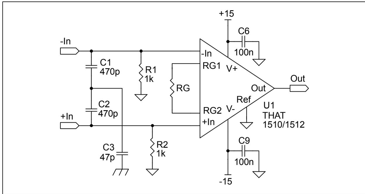
Figure 3. Basic 1510 / 1512 Circuit
