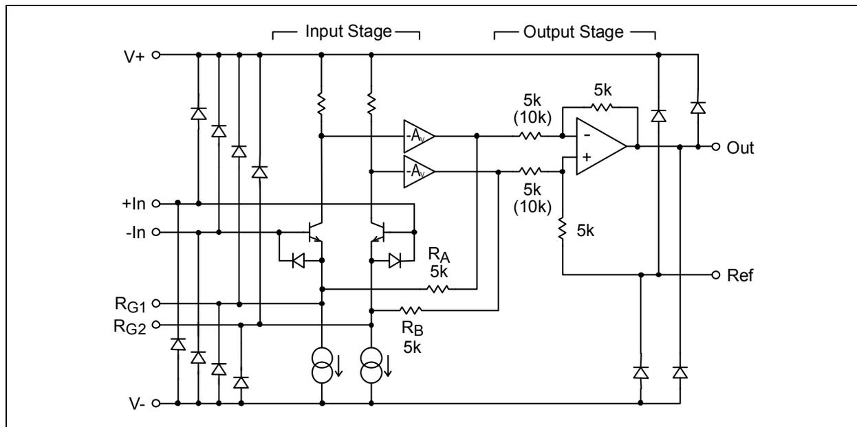
Figure 2. THAT 1510 / 1512 Equivalent Circuit with Protection Diodes
