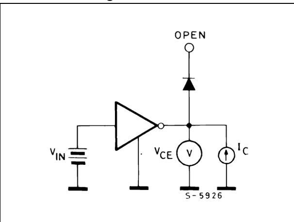
Figure 5. Collector-emitter saturation voltage Figure 6. Input current (ON)
