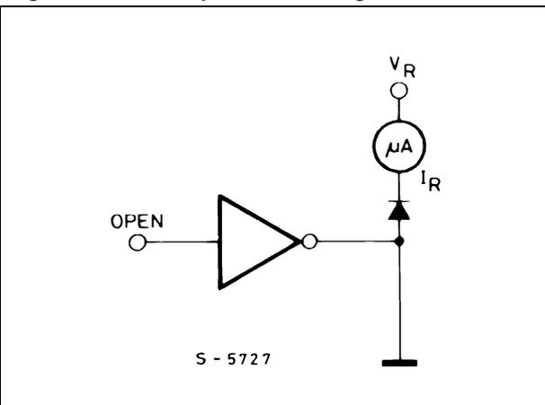
Figure 9. Clamp diode forward voltage
