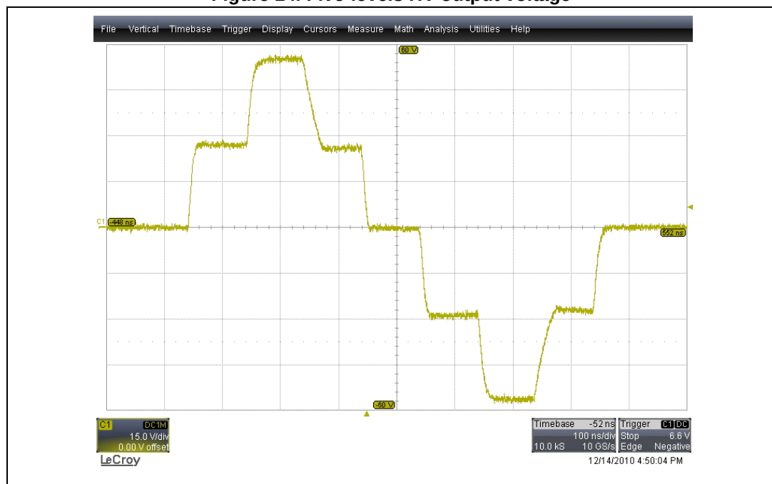
Figure 14. Five-levels HV output voltage
