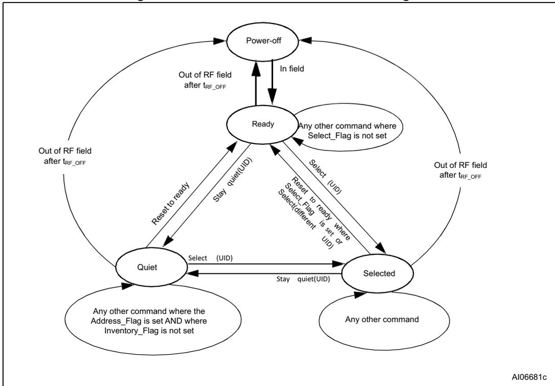
1. The M24LR16E-R returns to the Power Off state if the tag is out of the RF field for at least  $t_{RF\_OFF}$ . Please refer to application note AN4125 for more information.
