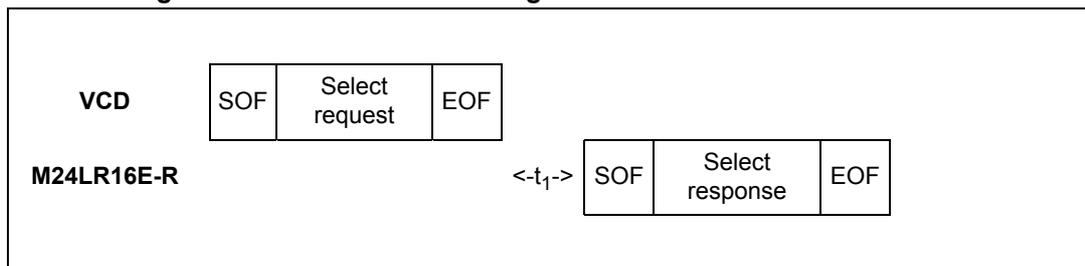
When configured in the RF busy mode, the RF WIP/BUSY pin is tied to 0 from the SOF that starts the Select command to the end of the M24LR16E-R response.
