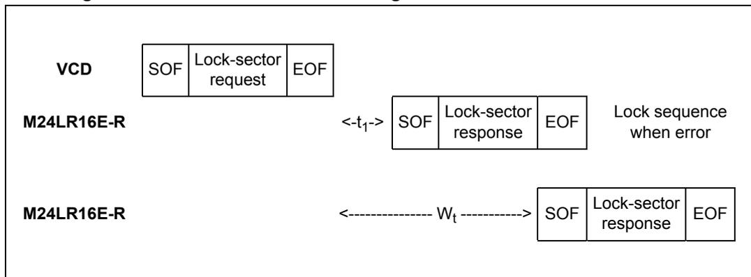
When configured in the RF busy mode, the RF WIP/BUSY pin is tied to 0 from the SOF that starts the Lock-sector command to the end of the M24LR16E-R response.
