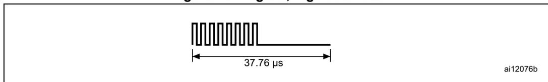
For the fast commands, a logic 0 starts with four pulses at 423.75 kHz ( $f_C/32$ ) followed by an unmodulated time of 9.44  $\mu$ s, as shown in [Figure 24](#).
