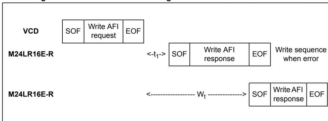
When configured in the RF busy mode, the RF WIP/BUSY pin is tied to 0 from the SOF that starts the Write AFI command to the end of the M24LR16E-R response.
