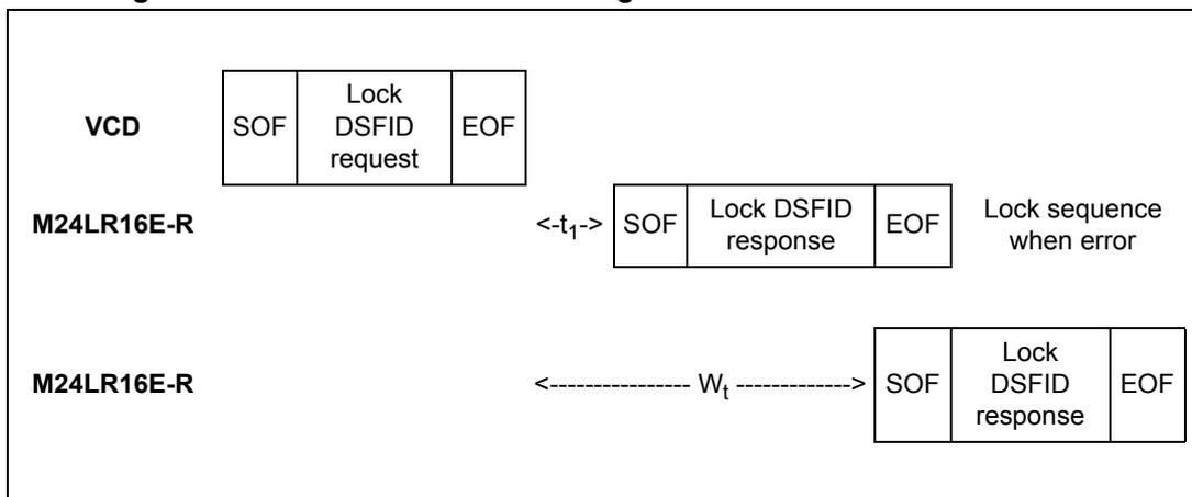
When configured in the RF busy mode, the RF WIP/BUSY pin is tied to 0 from the SOF that starts the Lock DSFID command to the end of the M24LR16E-R response.
