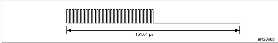
For the Fast commands, a logic 0 starts with 16 pulses at 423.75 kHz ( $f_C/32$ ) followed by an unmodulated time of 37.76  $\mu$ s, as shown in [Figure 28](#).
