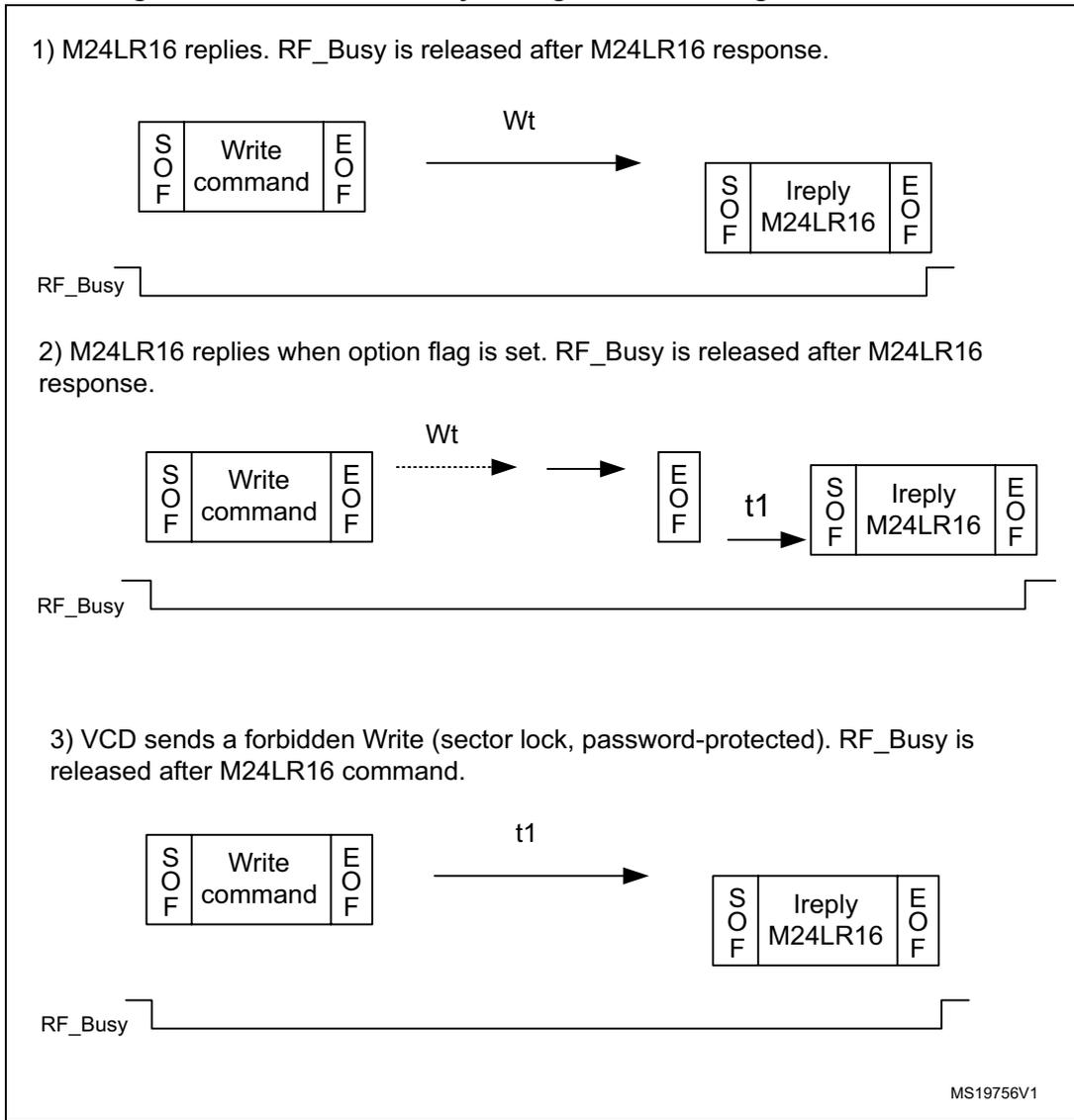
When configuring in the RF Write in progress mode, the RF WIP/BUSY pin is tied to 0 during the Write & verify sequence, as shown in [Figure 57](#).
