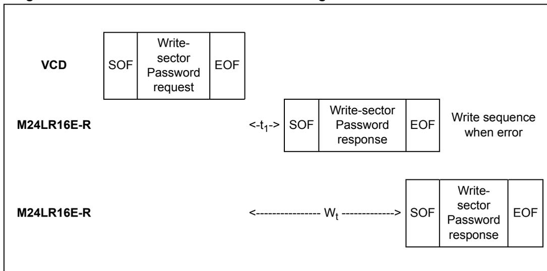
When configured in the RF busy mode, the RF WIP/BUSY pin is tied to 0 from the SOF that starts the Write-sector Password command to the end of the M24LR16E-R response.
