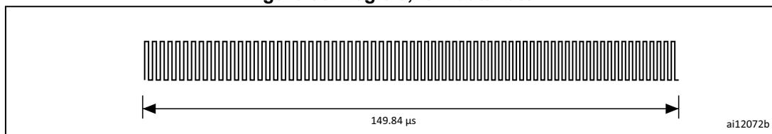
A logic 1 starts with 36 pulses at 484.28 kHz ( $f_C/28$ ) followed by 32 pulses at 423.75 kHz ( $f_C/32$ ) as shown in [Figure 34](#). Bit coding using two subcarriers is not supported for the Fast commands.
