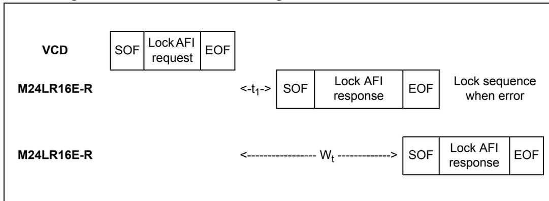
When configured in the RF busy mode, the RF WIP/BUSY pin is tied to 0 from the SOF that starts the Lock AFI command to the end of the M24LR16E-R response.
