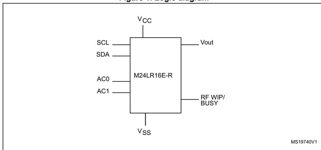
I<sup>2</sup>C uses a two-wire serial interface, comprising a bidirectional data line and a clock line. The devices carry a built-in 4-bit device type identifier code (1010) in accordance with the I<sup>2</sup>C bus definition.
