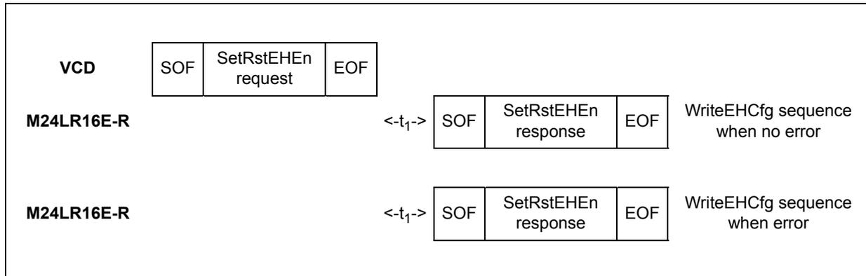
When configured in the RF busy mode, the RF WIP/BUSY pin is tied to 0 from the SOF that starts the SetRstEHEn command to the end of the M24LR16E-R response.
