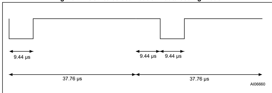
Figure 22. EOF for either data coding mode
