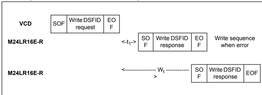
When configured in the RF busy mode, the RF WIP/BUSY pin is tied to 0 from the SOF that starts the Write DSFID command to the end of the M24LR16E-R response.
