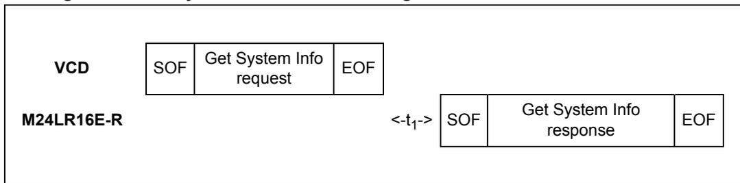
When configured in the RF busy mode, the RF WIP/BUSY pin is tied to 0 from the SOF that starts the Get System Info command to the end of the M24LR16E-R response.
