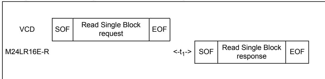
When configured in the RF busy mode, the RF WIP/BUSY pin is tied to 0 from the SOF that starts the Read Single Block command to the end of the M24LR16E-R response.
