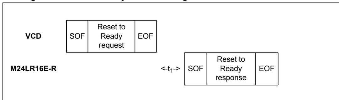
When configured in the RF busy mode, the RF WIP/BUSY pin is tied to 0 from the SOF that starts the Reset to ready command to the end of the M24LR16E-R response.
