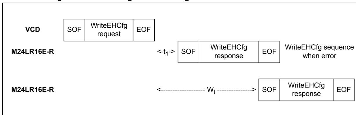
When configured in the RF busy mode, the RF WIP/BUSY pin is tied to 0 from the SOF that starts the WriteEHCfg command to the end of the M24LR16E-R response.
