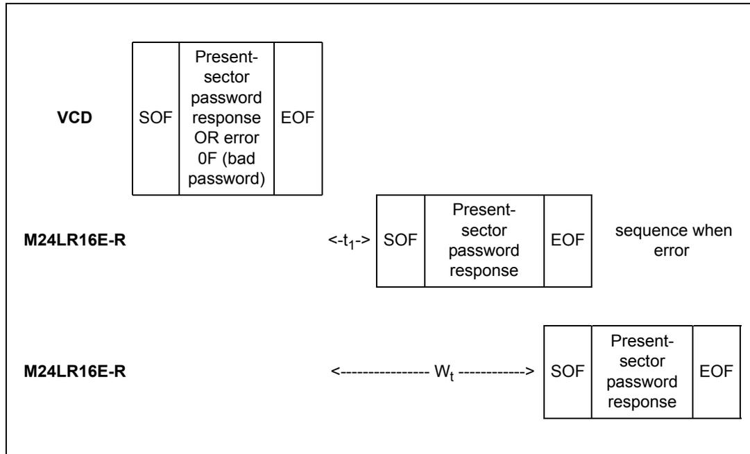
When configured in the RF busy mode, the RF WIP/BUSY pin is tied to 0 from the SOF that starts the Present Sector Password command to the end of the M24LR16E-R response.
