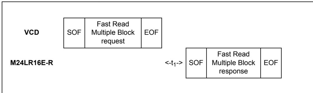
When configured in the RF busy mode, the RF WIP/BUSY pin is tied to 0 from the SOF that starts the Fast Read Multiple Block command to the end of the M24LR16E-R response.
