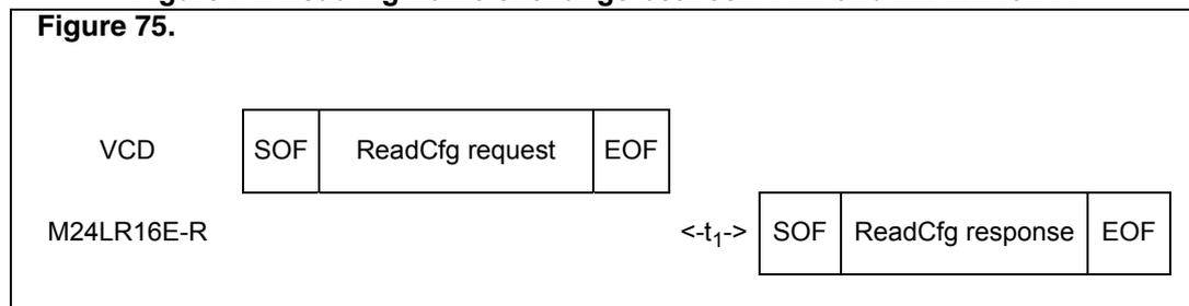
When configured in the RF busy mode, the RF WIP/BUSY pin is tied to 0 from the SOF that starts the ReadCfg command to the end of the M24LR16E-R response.
