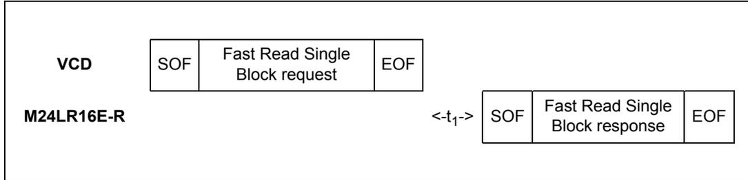
When configured in the RF busy mode, the RF WIP/BUSY pin is tied to 0 from the SOF that starts the Fast Read Single block command to the end of the M24LR16E-R response.
