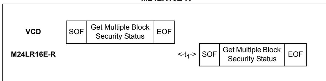
When configured in the RF busy mode, the RF WIP/BUSY pin is tied to 0 from the SOF that starts the Get Multiple Block Security Status command to the end of the M24LR16E-R response.
