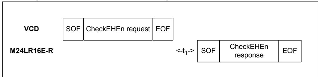
When configured in the RF busy mode, the RF WIP/BUSY pin is tied to 0 from the SOF that starts the CheckEHEn command to the end of the M24LR16E-R response.
