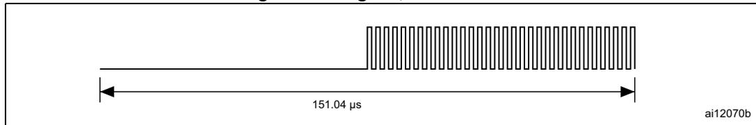
For the Fast commands, a logic 1 starts with an unmodulated time of 37.76  $\mu$ s followed by 16 pulses at 423.75 kHz ( $f_C/32$ ), as shown in [Figure 30](#).
