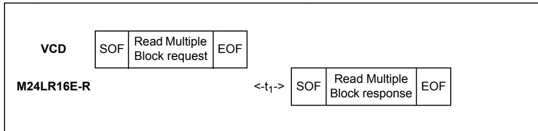
When configured in the RF busy mode, the RF WIP/BUSY pin is tied to 0 from the SOF that starts the Read Multiple Block command to the end of the M24LR16E-R response.
