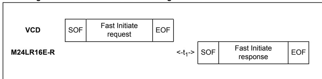
When configured in the RF busy mode, the RF WIP/BUSY pin is tied to 0 from the SOF that starts the Fast Initiate command to the end of the M24LR16E-R response.
