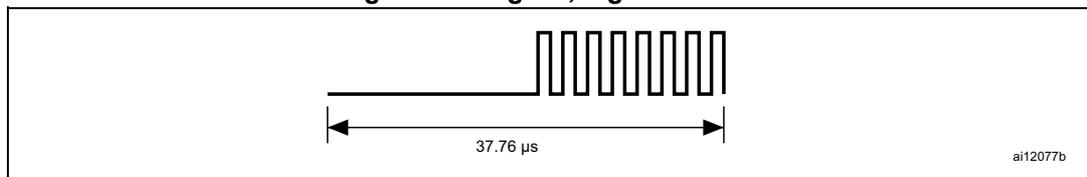
For the Fast commands, a logic 1 starts with an unmodulated time of 9.44  $\mu$ s followed by four pulses of 423.75 kHz ( $f_C/32$ ), as shown in [Figure 26](#).
