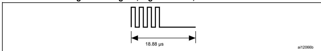
A logic 1 starts with an unmodulated time of 18.88  $\mu$ s followed by eight pulses at 423.75 kHz ( $f_C/32$ ), as shown in [Figure 25](#).
