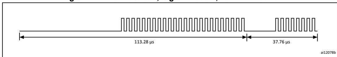
For the Fast commands, the SOF comprises an unmodulated time of 28.32  $\mu\text{s}$ , followed by 12 pulses at 423.75 kHz ( $f_C/32$ ), and a logic 1 that consists of an unmodulated time of 9.44  $\mu\text{s}$  followed by four pulses at 423.75 kHz, as shown in [Figure 36](#).
