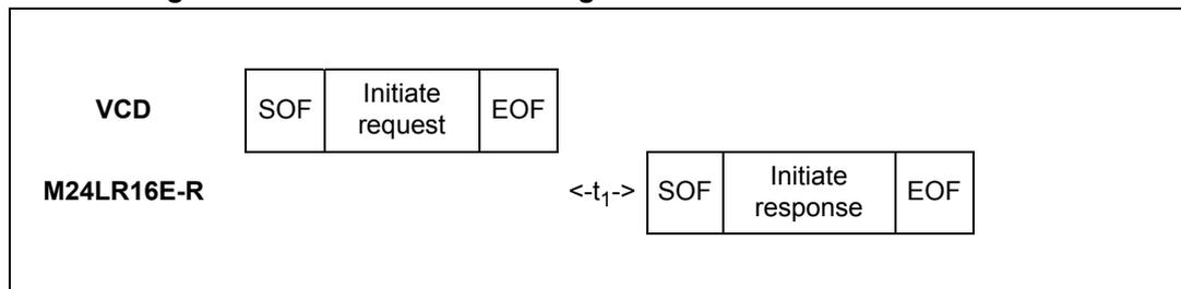
When configured in the RF busy mode, the RF WIP/BUSY pin is tied to 0 from the SOF that starts the Initiate command to the end of the M24LR16E-R response.
