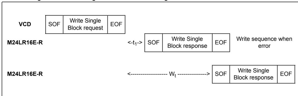
When configured in the RF busy mode, the RF WIP/BUSY pin is tied to 0 from the SOF that starts the Write Single Block command to the end of the M24LR16E-R response.
