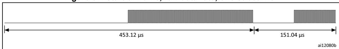
For the Fast commands, the SOF comprises an unmodulated time of 113.28  $\mu\text{s}$ , followed by 48 pulses at 423.75 kHz ( $f_C/32$ ), and a logic 1 that includes an unmodulated time of 37.76  $\mu\text{s}$  followed by 16 pulses at 423.75 kHz, as shown in [Figure 38](#).
