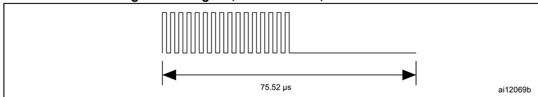
A logic 1 starts with an unmodulated time of 75.52  $\mu$ s followed by 32 pulses at 423.75 kHz ( $f_C/32$ ), as shown in [Figure 29](#).
