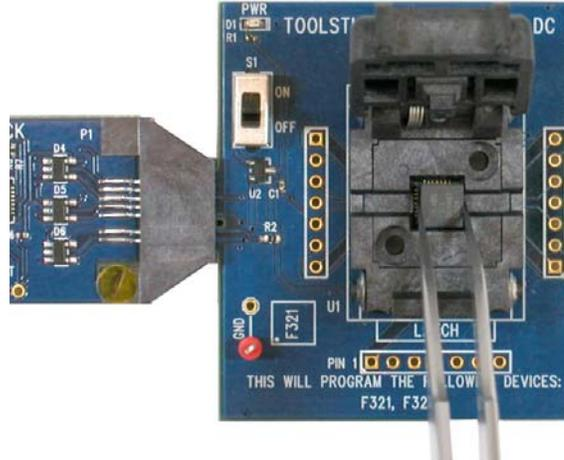
**Figure 16. Removing a Device from a Clam-Shell Socket**
