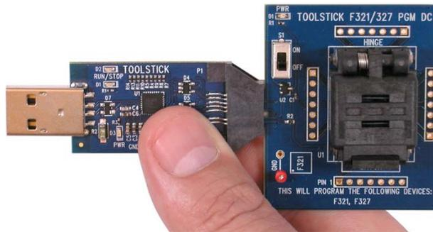
Figure 2. Improper Method of Holding the ToolStick
