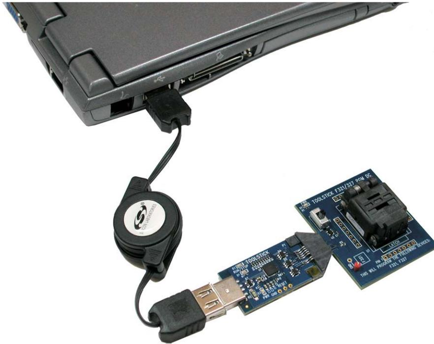
Figure 5. ToolStick Socket Platform Connected to PC
