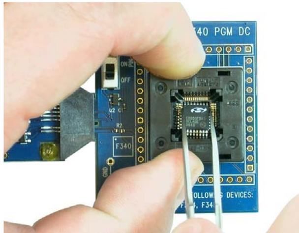
**Figure 17. Removing a Device from a Top-loading Socket**
