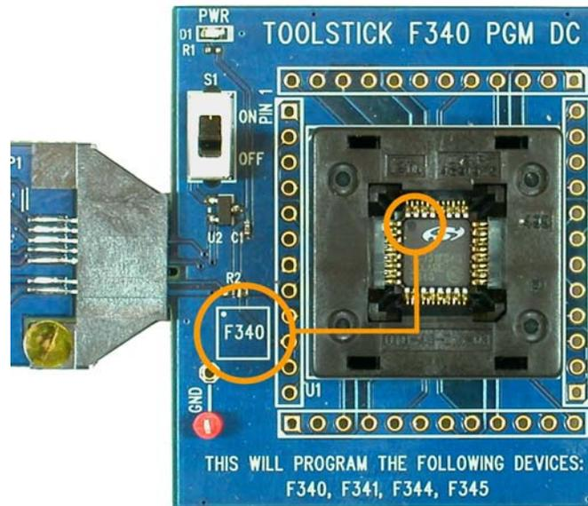
**Figure 7. Socket Orientation**
