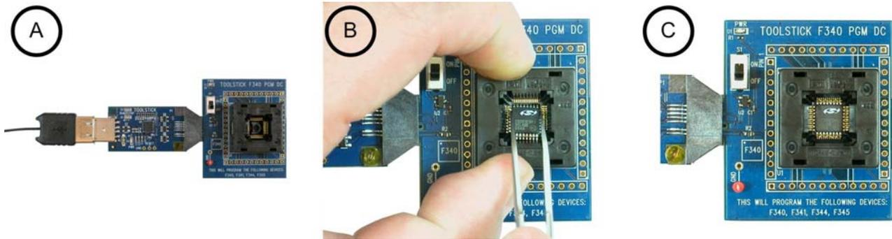
**Figure 9. Top-loading Socket**
