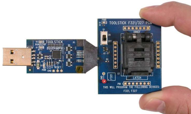
Figure 1. Proper Method of Holding the ToolStick
