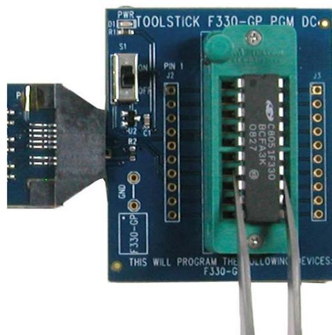
**Figure 18. Removing a Device from a ZIF Socket**
