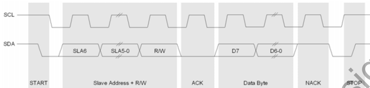
Figure 12. I²C Bit Timing Diagram
