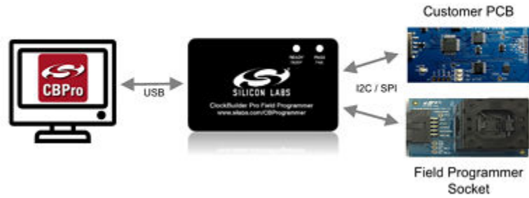
Figure 4.1. PC to CBPROG-DONGLE Connection
