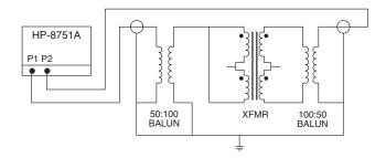
5. Crosstalk Attenuation — In the dual packages, which contain transmit and receive transformers side by side, sufficient crosstalk attenuation is achieved by the inherent characteristics of the toroid cores as well as by their proper positioning. The crosstalk attenuation is typically 50 dB or better from 100 KHz to 10 MHz. This result was established with the test circuit shown below.
