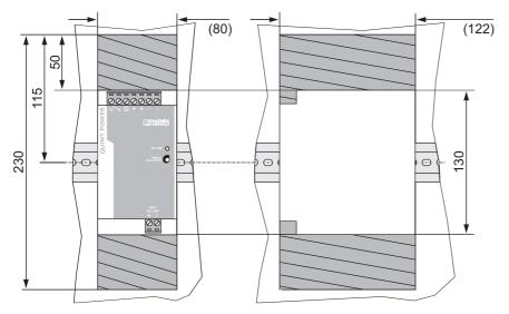
Slim-style installation: Installation depth 125 mm (+ DIN rail) (state at delivery) Low-profile installation: Installation depth 83 mm (+ DIN rail)
