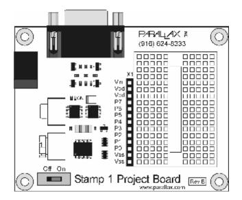
For permanent projects, you may leave off the breadboard and solder components directly to the PCB. Parallax offers a range of accessory component kits for the BS1 Project Board. The figure below shows the layout of the printed circuit board:
