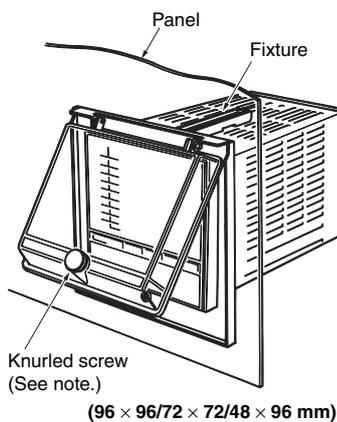
**Note:** Tighten the knurled screw to a torque of 0.02 N·m and the hexagonal nut to a torque of 0.05 N·m.
