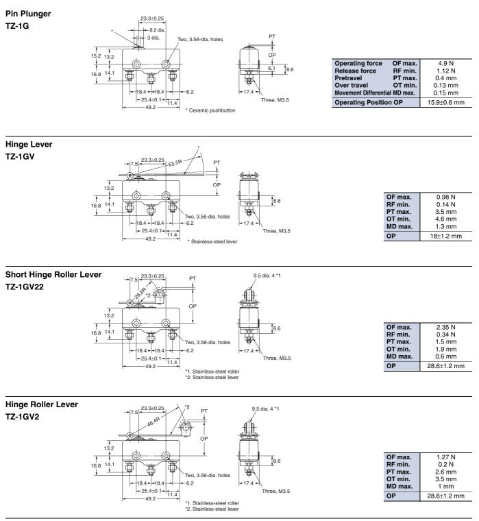
Note: Each dimension has a tolerance of  $\pm 0.4$  mm unless otherwise specified.
