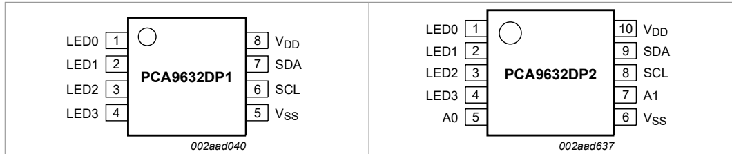
Figure 2. Pin configuration for TSSOP8
