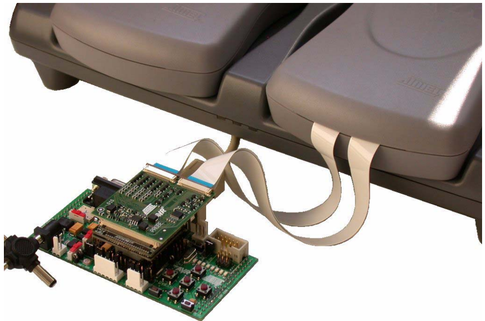
Figure 3-46 . Connecting AVR ICE 50 for Debugging
