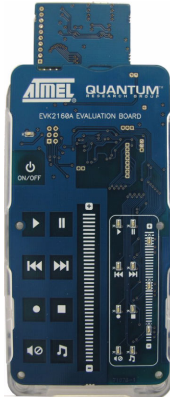
Figure 1-6. USB Plug-in Card and EVK2160A Setup Complete
