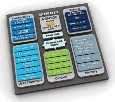
Backup unit with RTC, timer and four 32-bit registers and fast wake-up
