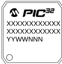
100-Lead TQFP (12x12x1 mm)
