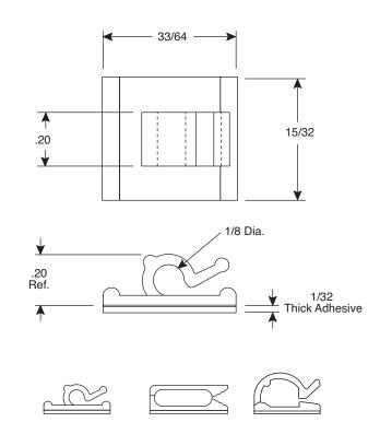
EPD Adhesive backed nylon wire and cable clips are used to route wires and cables. The parts are backed with polyethylene foam tape, and feature a releasable clip so wires can be removed after assembly if desired. Parts are stocked in natural. When ordering black parts, add the letter "B" to the end of the part number.
