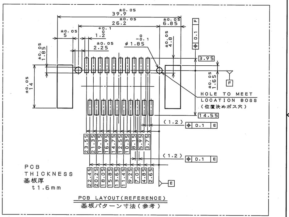
NOTE 1. THE COPLANARITY TERMINALS, INCLUDING THE HOLD-DOWNS, SHALL BE 0.15 MAX AS REFERENCED FROM THE SURFACE PLATE. (REFERENCE FIGURE 1)
