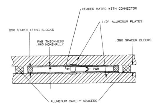
PWB'S MEASURE .365 OUTSIDE TO OUTSIDE AND ARE CLAMPED BETWEEN THE 1/2" ALUMINUM PLATES WITH SPACER BLOCKS MEASURING .380.
