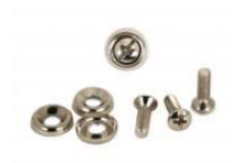
The 1421 screw provides a standard 0.625" rack screws length with 10-32 threads. The screw itself features a slotted oval head and has a nickel plate finish.
