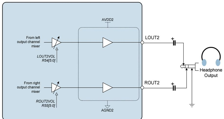
**Figure 28 LOUT2 and ROUT2 Class AB Headphone Configuration**
