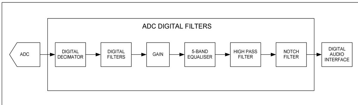
Figure 19 ADC Digital Filter Path
