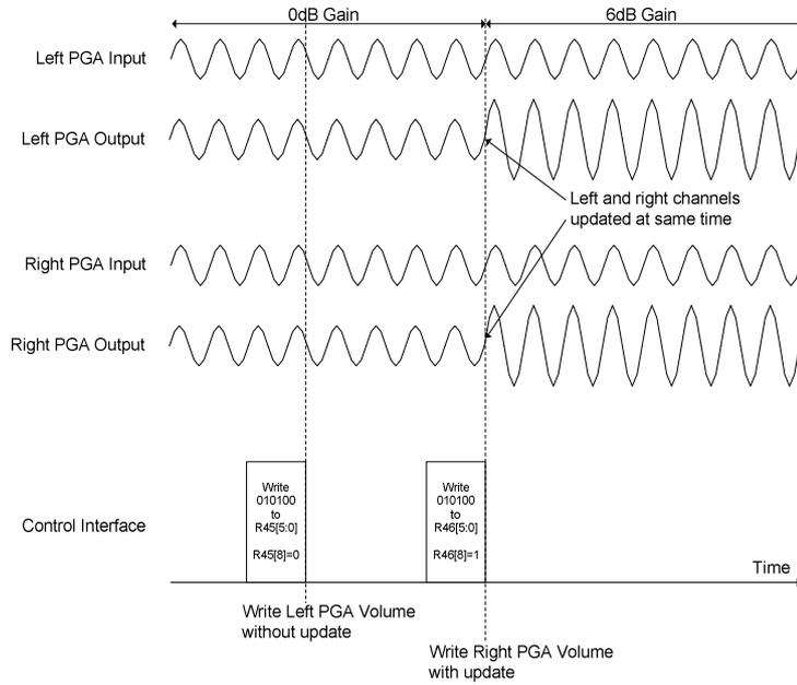
**Figure 13 Simultaneous Left and Right Volume Updates**
