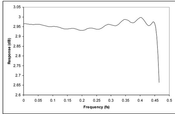
**Figure 42 DAC Digital Filter Ripple (128xOSR)**
