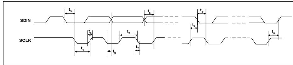
Figure 6 Control Interface Timing – 2-Wire Serial Control Mode
