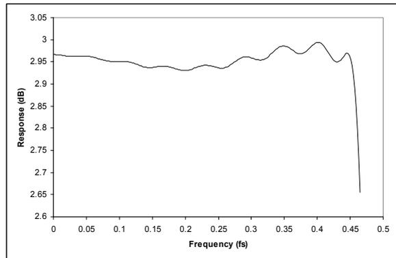
**Figure 44 DAC Digital Filter Ripple (64xOSR)**
