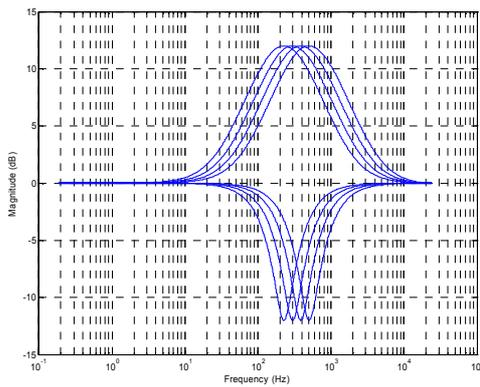
Figure 53 EQ Band 2 – Peak Filter Centre Frequencies, EQ2BW=0
