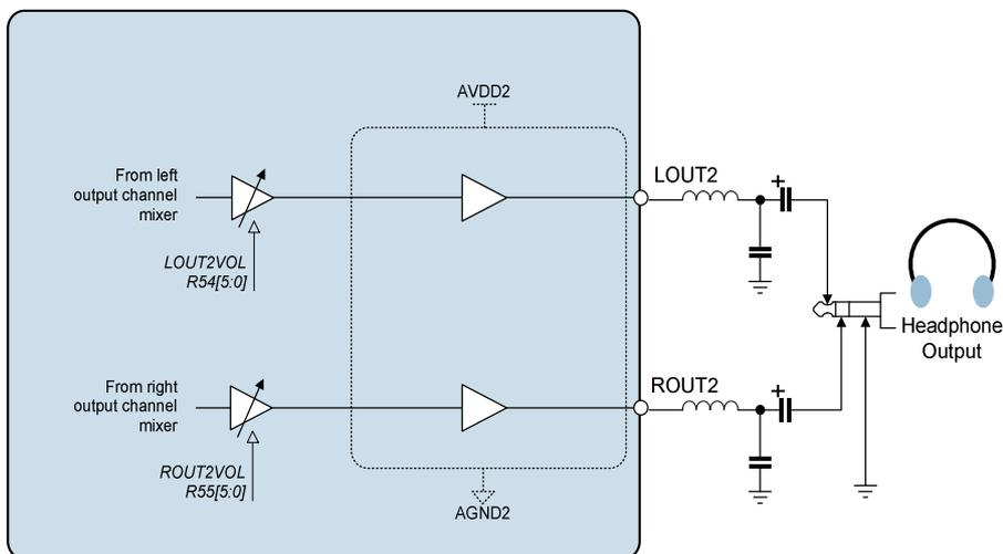
**Figure 27 LOUT2 and ROUT2 Class D Headphone Configuration**
