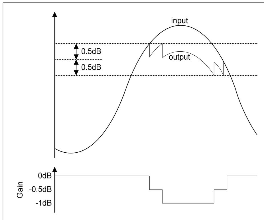
**Figure 24 DAC Digital Limiter Operation**
