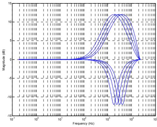
Figure 59 EQ Band 4 – Peak Filter Centre Frequencies, EQ3BW=0
