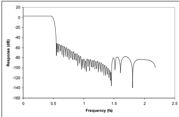
**Figure 41 DAC Digital Filter Frequency Response (128xOSR)**
