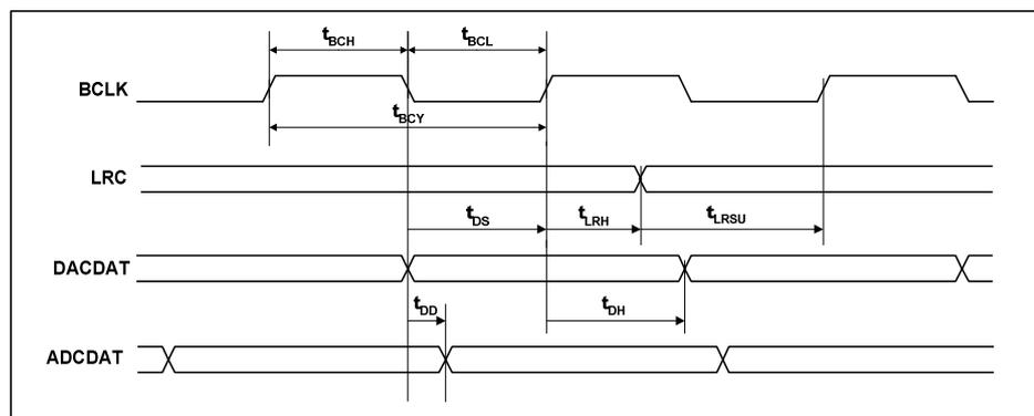
Figure 4 Digital Audio Data Timing – Slave Mode
