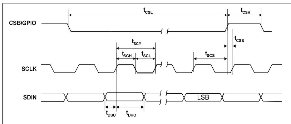
Figure 5 Control Interface Timing – 3-Wire Serial Control Mode
