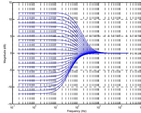
Figure 52 EQ Band 1 Gains for Lowest Cut-off Frequency
