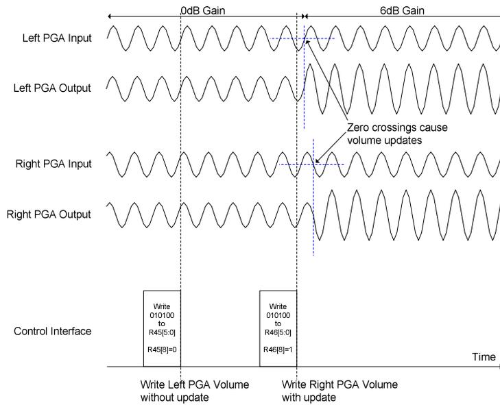
**Figure 15 Volume Update using Zero Cross Detection**
