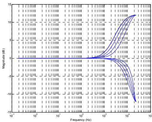
Figure 62 EQ Band 5 High Frequency Shelf Filter Cut-offs
