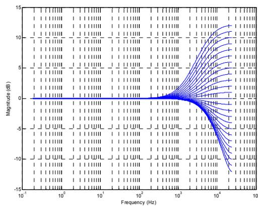
Figure 63 EQ Band 5 Gains for Lowest Cut-off Frequency
