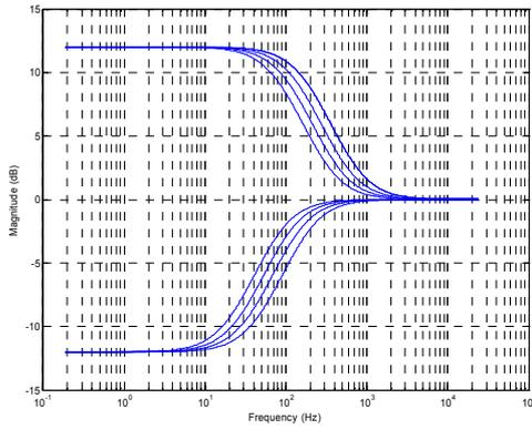
Figure 51 EQ Band 1 Low Frequency Shelf Filter Cut-offs
